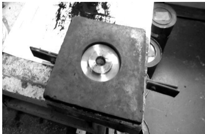
Fig.3 Placement of the knife blank in graphite form
